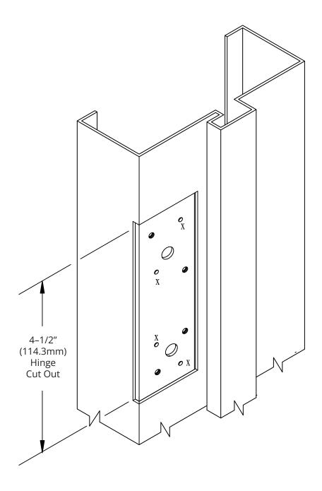
4 Projection dimpled marked (X) are added to hinge reinforcement for standard 4–1/2" x 4–1/2" full mortised template hinge .134 thickness.
