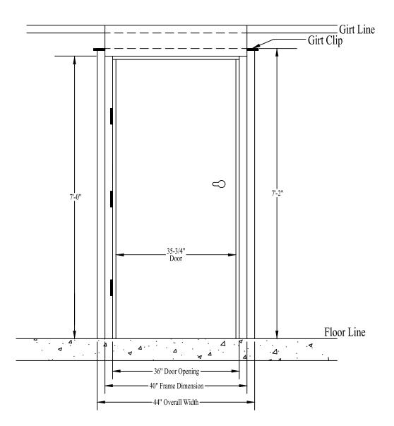
3070 Standard Preassembled Door Includes The Following Components:
