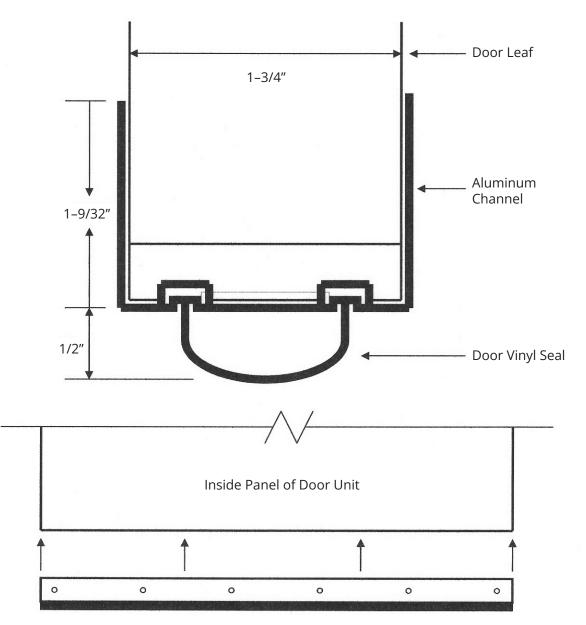
Door Bottom Seal Aluminum Channel is Installed with Screws to the Inside Skin of the Door Leaf to Prevent Corrosion
