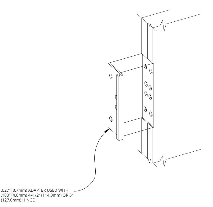
WHEN ATTACHING ADAPTER, THIS WILL CAUSE A 1/4" (6.4MM) BRACKET
